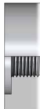
BSPP female port (spot-faced)
