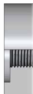
BSPP female port (spot-faced)
