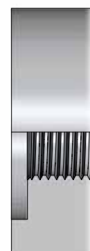
BSPP female port (spot-faced)
