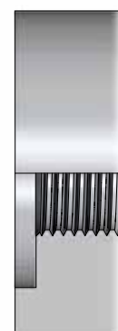
BSPP female port (spot-faced)
